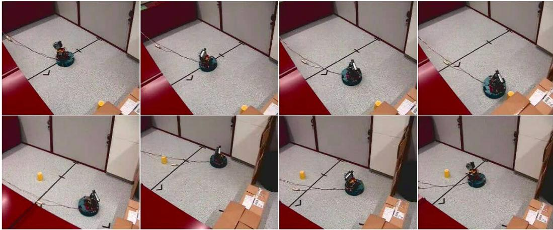
Fig. 3. Snapshots (ordered like text) of robot moving around inside the fenced area containing the target object, a yellow cup. Top row: after approximately 20 minutes of learning, the robot searches for the target object effectively, and approaches it directly. Bottom row: the robot generalizes successfully to novel starting positions and target object positions.
